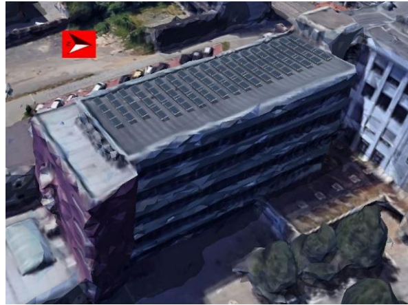
Figure 4. Detail of 3D model created in PIX4D (building)
