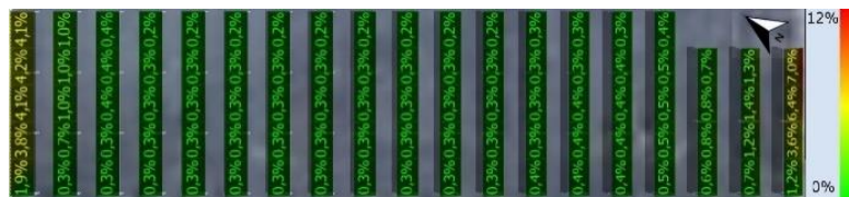
Figure 5. Shading simulation of PVSOL model
