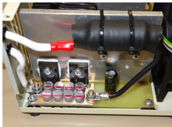
Figure 3. Output synchronous rectifier, filtering capacitors, inrush limiting inductor (top).
