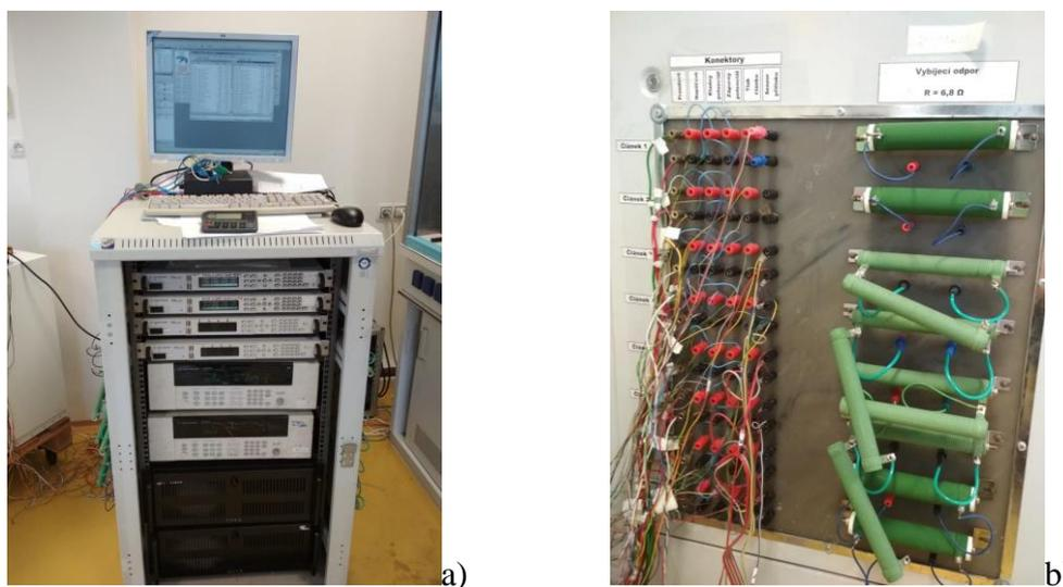
**Figure 1.** a) Measuring control panel; b) Terminal blocks and discharge resistors on the side of the measuring control panel
