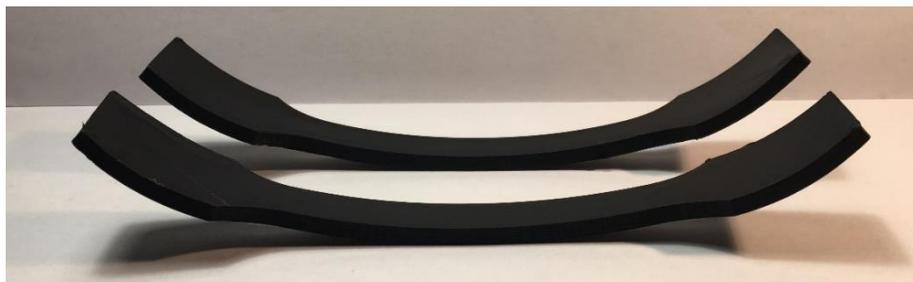
**Figure 2.** Example of an unannealed testing bodies
