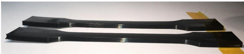
**Figure 3.** Example of an annealed testing bodies at 80 ° C
