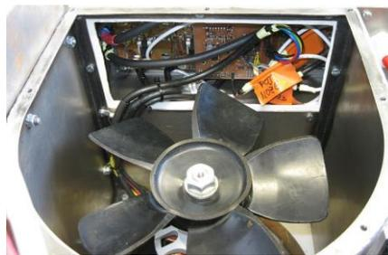
*Figure 3. Inside space of the dustproof cover of the knife motor.*
