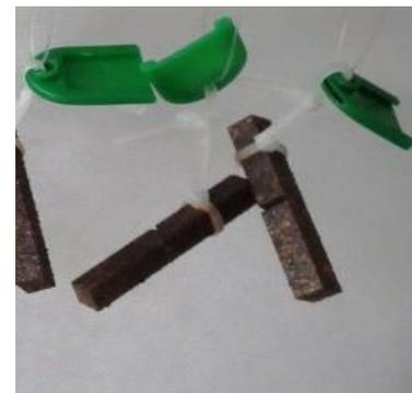
**Figure 1a.** Set A samples after 9 cycles of corrosion test
