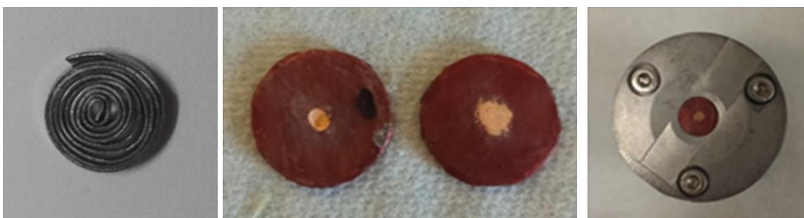
**Figure 1.** Counter-electrode (left), Pasted negative electrode (center), assembled in-situ cell for laser confocal microscopy (right)
