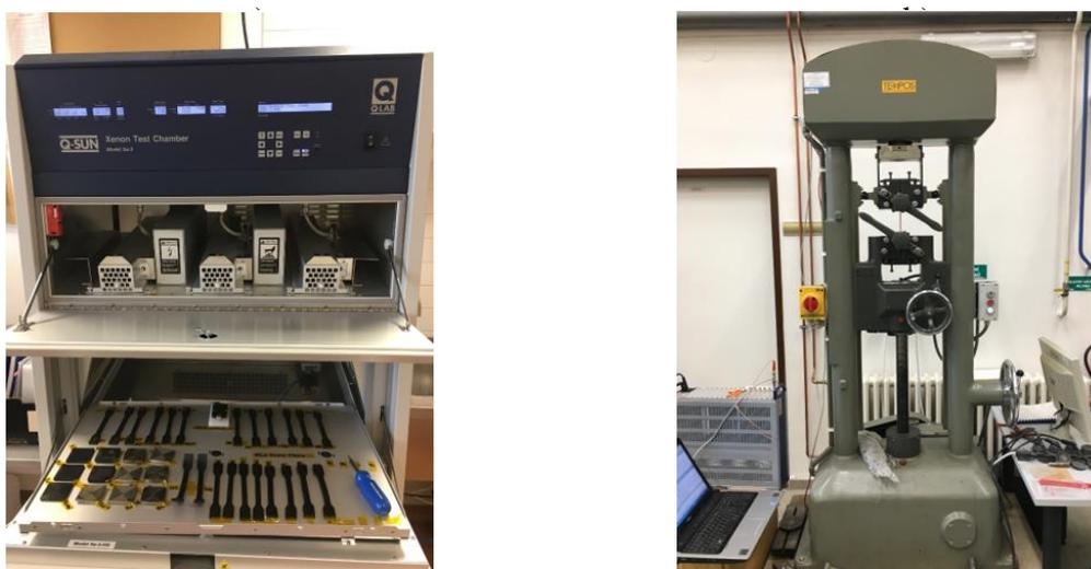
**Figure 1.** a) Climatic chamber Q-SUN-Xe3, b) TEMPOS ZD20/200 kN
