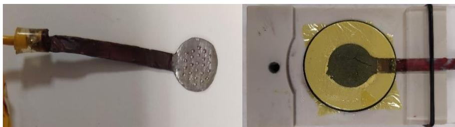
**Figure 1.** On the left, there is a picture of the detail of the lead substrate. On the right, there is a picture of the complete test electrode covered with polyamide foil.
