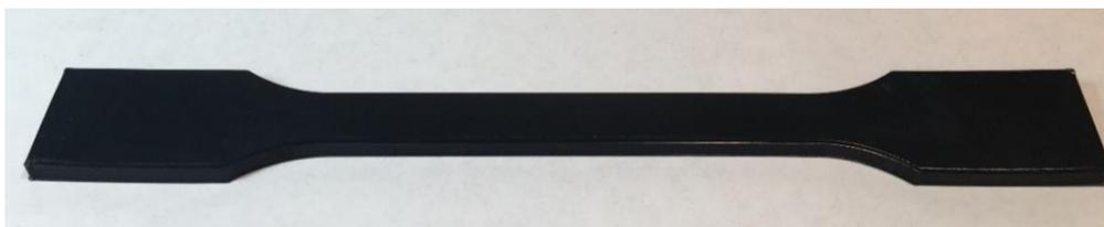
**Figure 4.** Example of an annealed testing body at 100 ° C
