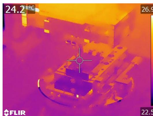
**Figure 2b.** Example of heat measurement at the friction point during the experiment, load 8 N (PTFE ball)
