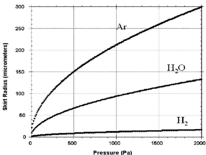
**Fig. 2** Beam broadening in ESEM (20 keV, 5 mm beam path length) [2]
