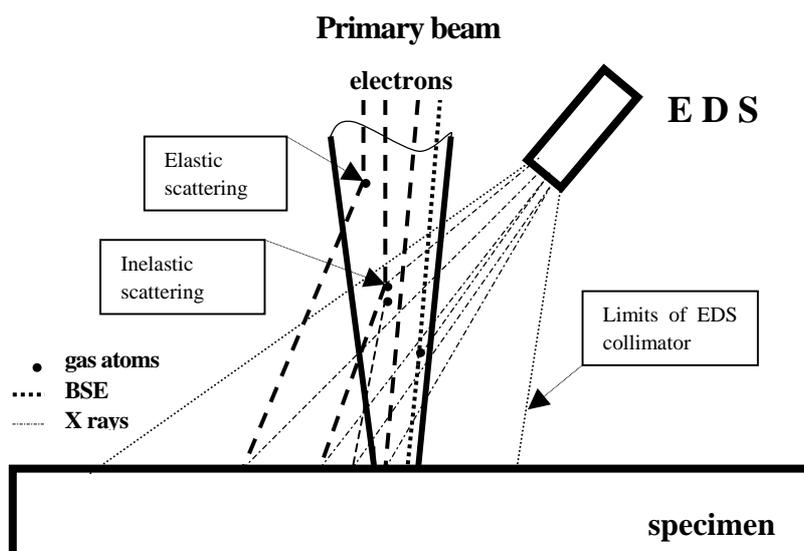
**Fig. 1** Electron scattering and X - rays collection
