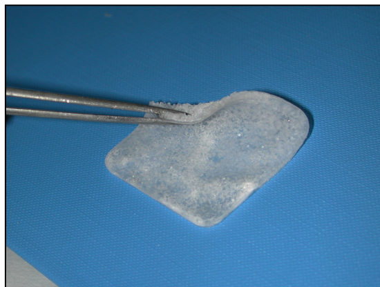
Fig. 1 Prepared elastic inorganic-organic phosphosilicate membrane exhibiting proton conductivity.
