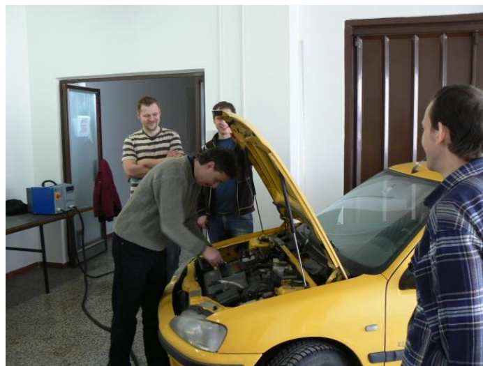
Fig. 5: Connection of the charger to the vehicle Peugeot 106 electric
