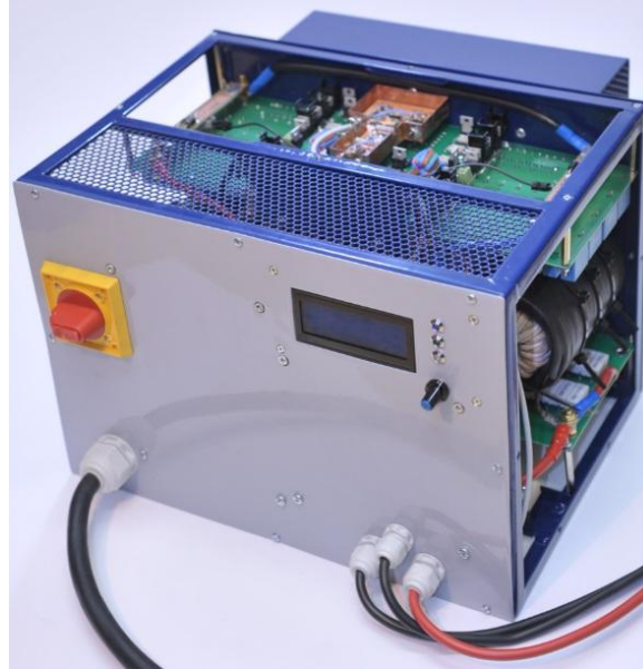
Fig. 5: Fast-charger RN16-380 (upper cover removed)
