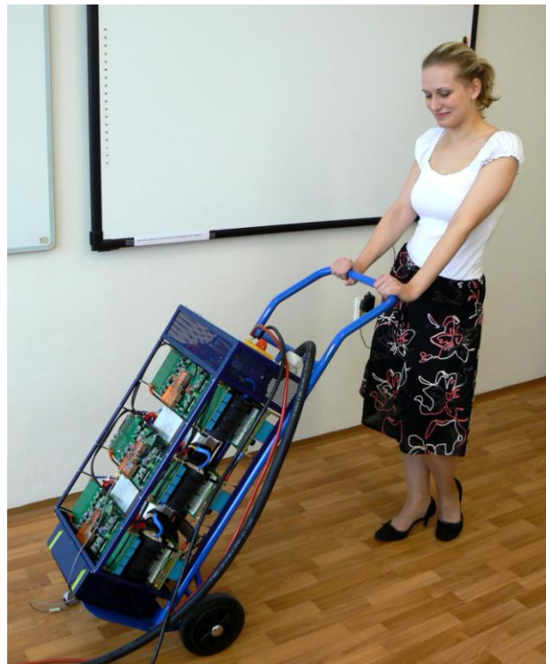
Fig. 6: Fast-charger RN48-480 (upper cover removed)
