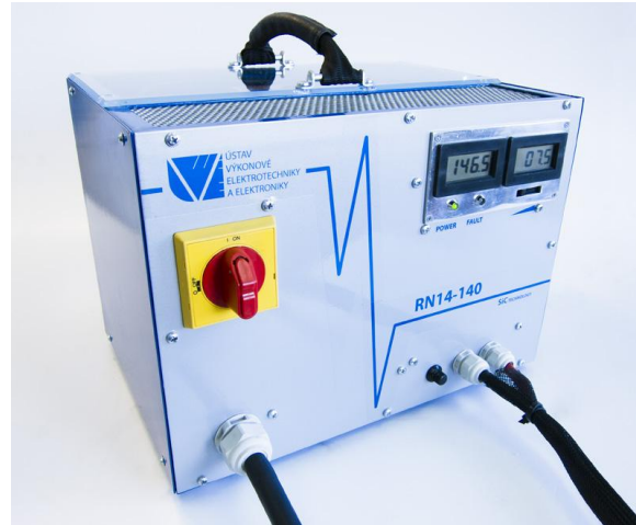
Fig. 2: Fast-charger RN14-140 (front view)
