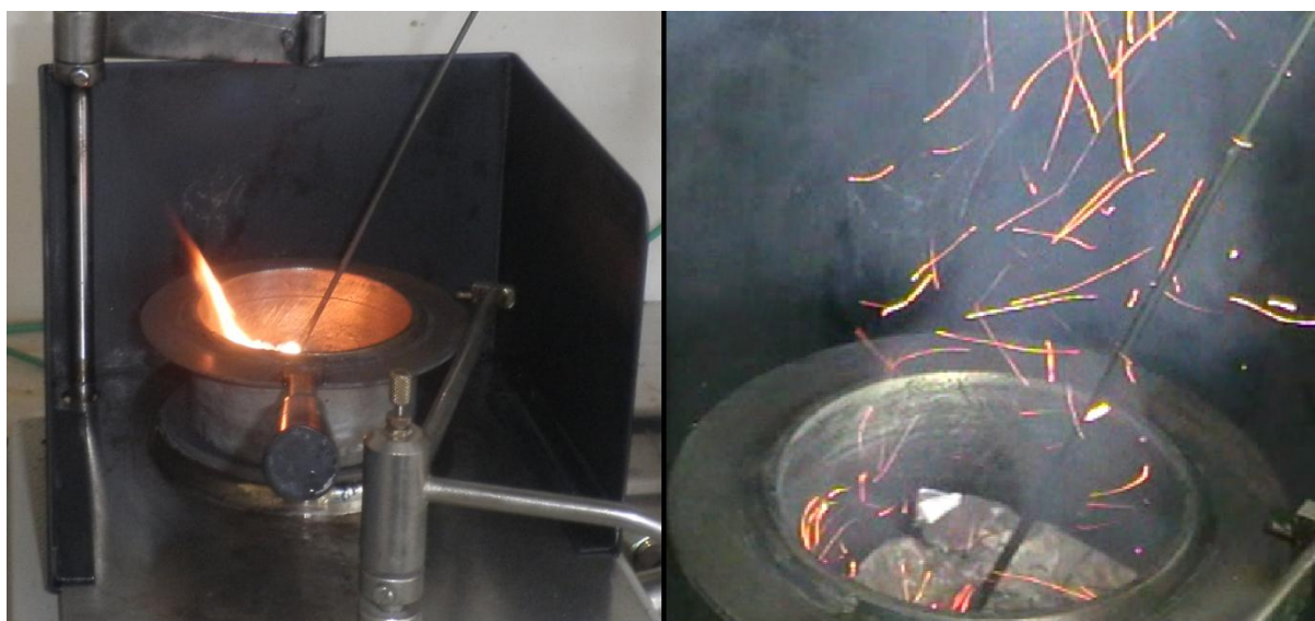
Fig. 9: Explosion of a LiClO 4 -containing gel in air at 450°C.
