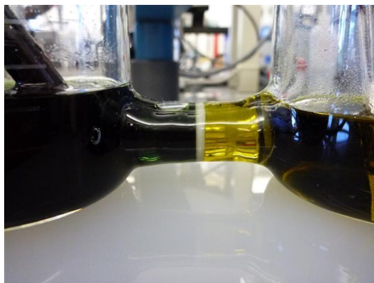
Fig. 5: Detail of the H-cell after extended electrolysis of a vanadium salt in 5 mol/l sulfuric acid (right side the reduced form, left the oxidized).
