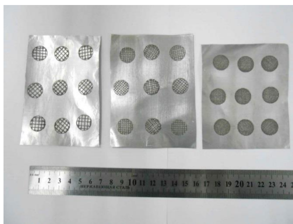
Figure 1. Samples of aluminum foil, the surface of which is modified by spectral purity graphite. Diameter of the modified surface is 16 mm. The aluminum current collectors have the different degree of modification. 1. Ten graphitized lines (lines intersect at an angle of 90°; 2. Sixteen graphitized lines; 3. Fully modified surface
