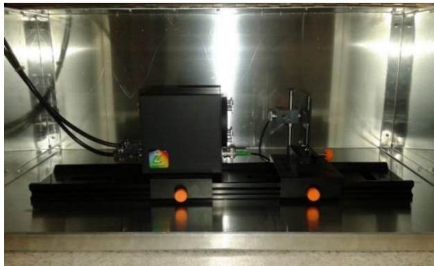
Figure 2. Light source and solar cell holder with light sensitive sensor.
