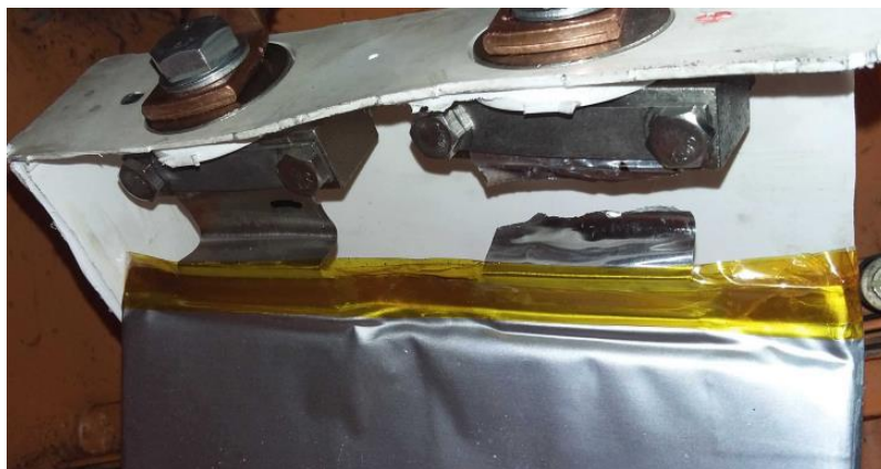
Figure 3. Cell view after short circuit on the terminals
